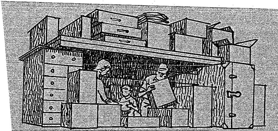
With doors, furniture and appliances, plus stacks of other shielding material, you can create an enclosure large enough to live in for a short time. If possible, use boxes filled with sand or earth as shielding material, and fill drawers and trunks with sand or earth.
