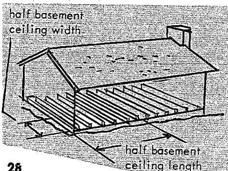
This is similar to Plan A, except that new extra joists are fitted into part of the basement ceiling to support the added weight of the shielding (instead of using a beam and a screwjack column).
